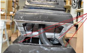
Attach the three solution tubes shown below.
